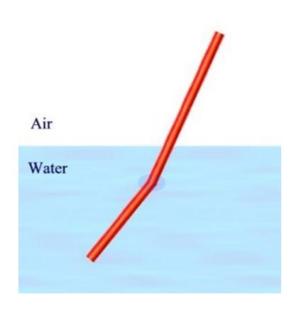
The bending of light rays as they pass between two different media is called refraction
